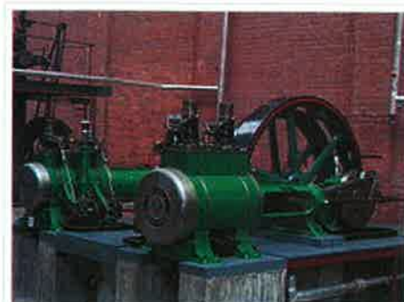
A Robey horizontal 'cross-compound' steam engine: the smaller, high-pressure cylinder is on the left; the larger, low-pressure cylinder on the right
